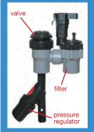
Irrigation valves are designed to work within a certain pressure range (pounds per square inch or psi) and flow range (gallons per minute or GPM). If you redesign your system and use low flow irrigation, the flow through the valve may be so low that your existing valve will not operate effectively and may get stuck in the "open" position, wasting water. If you have flow lower than 5 GPM per valve, check your valve specifications for flow range to determine whether or not to replace your valves.
